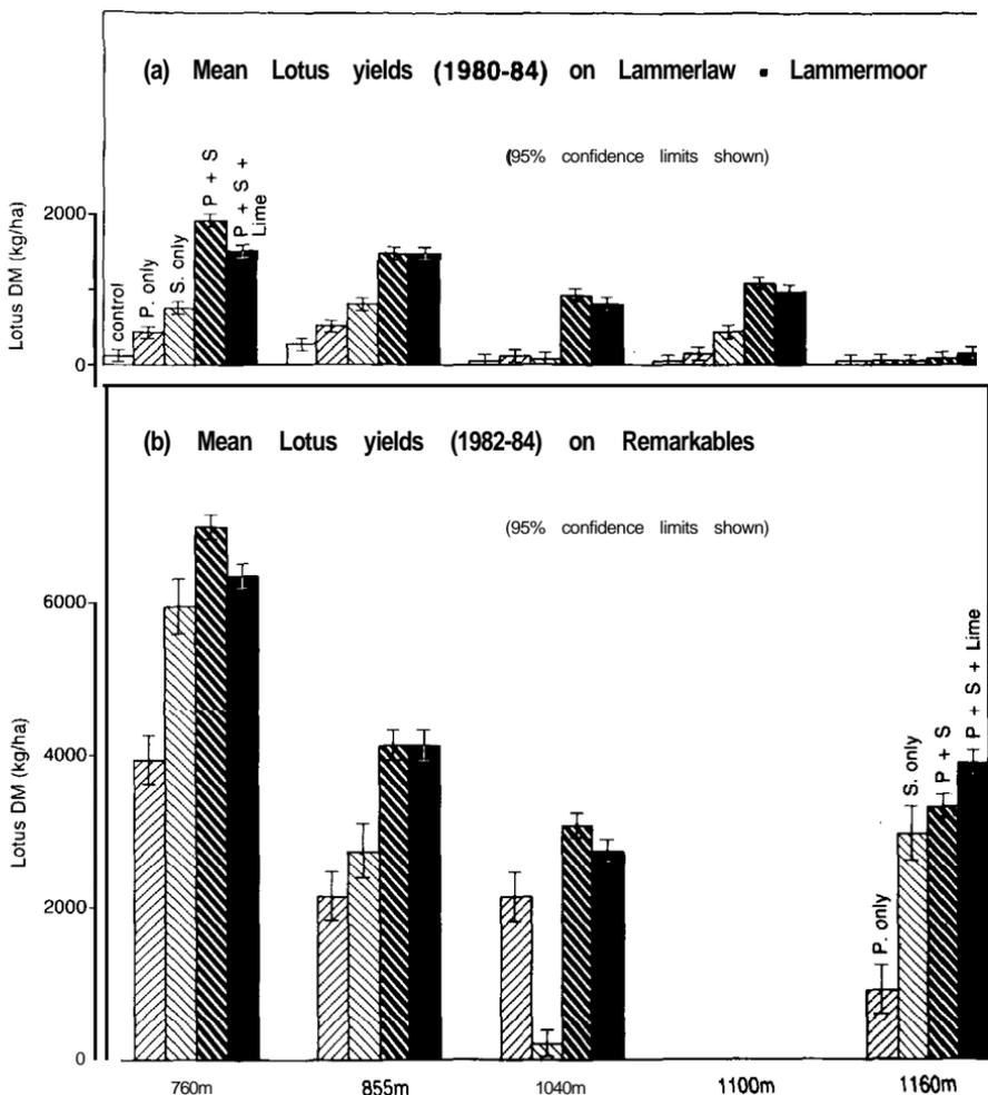
Figure 1: The effects of fertiliser treatments and altitude on mean annual yields of lotus on (a) lammerlaw-lammermoor ranges (1980-84) (b) Remarkables range (1982-84).
