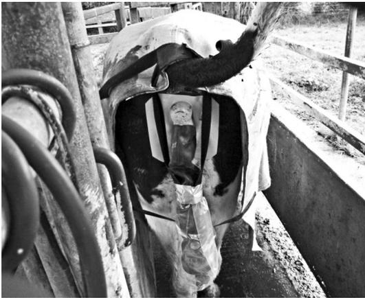
**Figure 1** AgResearch urine sensor (Mark II) on a dairy cow. Two long Velcro® straps hold the sensor onto the cow cover. The urine catcher is glued around the vulva and urine passes down a section of motorcycle inner tube to the urine sensor. A polythene sleeve covers the urine sensor to prevent faecal soiling. A PVC sheet, glued to the skin, prevents the straps levering the catcher from the skins, thereby allowing urine leakage.
