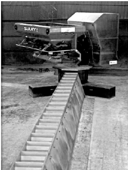
Figure 2 The CEMAGREF CEMIB automatic testing device. Reproduced from Piron et al. (2010).
