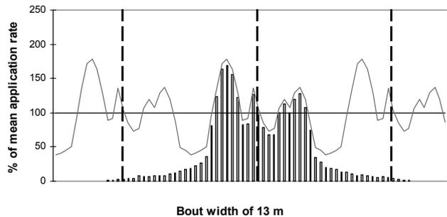
**Figure 3** Example of Type 2 spread pattern (CV 40%). Bars show single pass pattern, continuous line shows overlapped pattern, dashed vertical lines indicate bout width of spreader.
